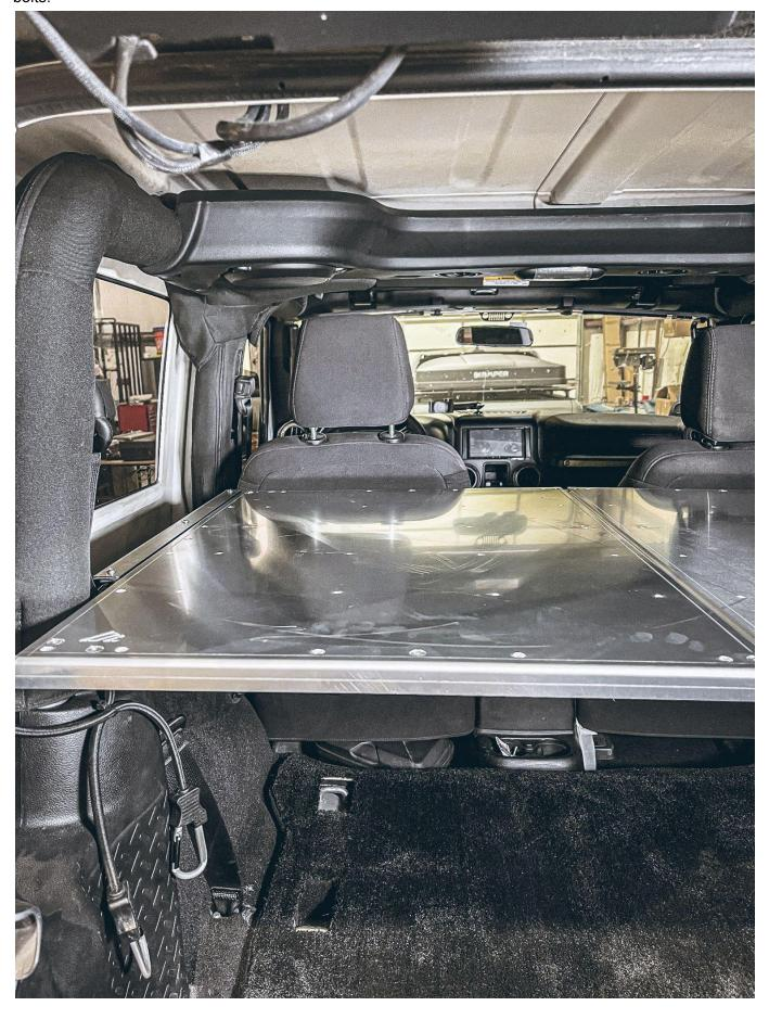
Once that is completed you can make sure the triangle support pieces are attached to the underside of those molle panel supports before installing the molle panel supports to the Jeep using the factory hardtop bolts using the M6 button head bolts.
