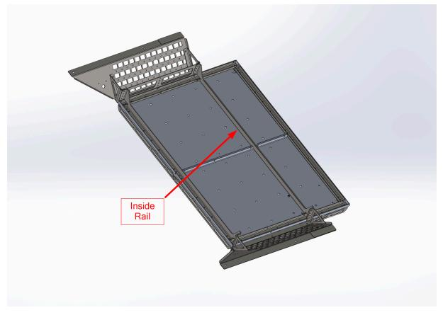
After that is done you will attach the 2 aluminum panels to the shelf frame using the provided M6 flat pan head bolts.
