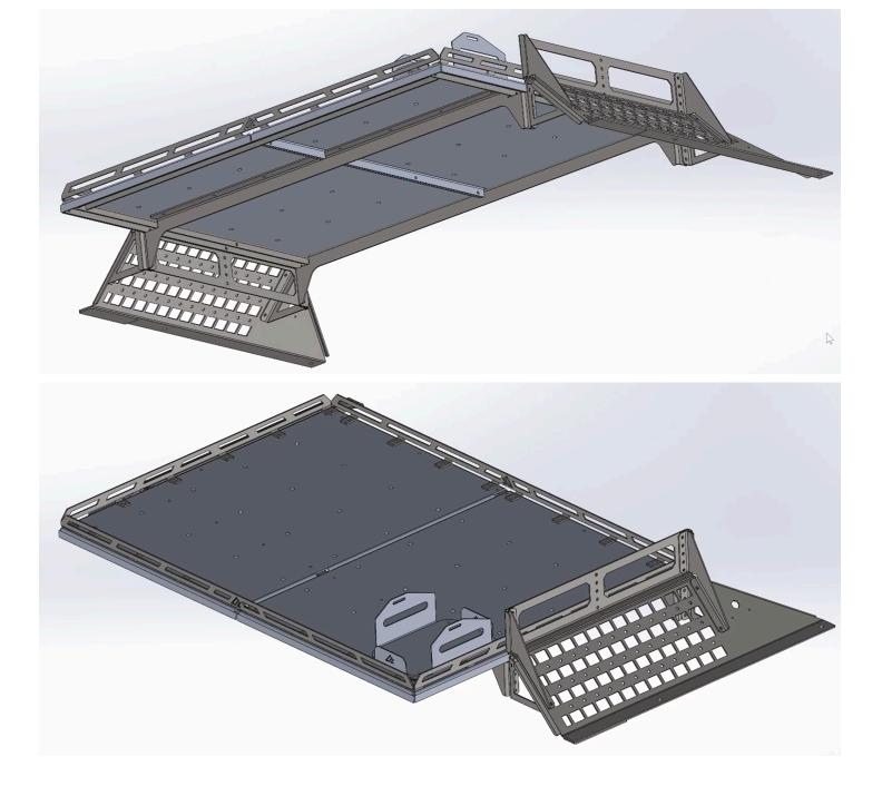
After that is done you can install your assembled shelf to the molle panels, tightening all of the screws and mount the edge guards using the provided M6 button head bolts. With that, you're all set!
